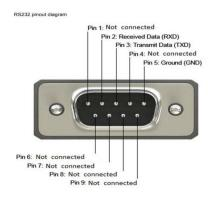
The port settings should always be 8 data bits, no parity and one stop bit. The baud rate is fixed at 115200 bits per second. All commands and responses are in ASCII form.
